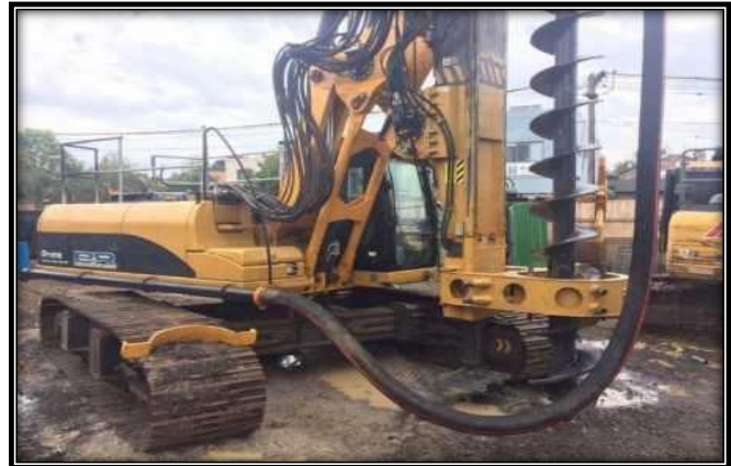
Figure 98 Pile Boring Equipment
